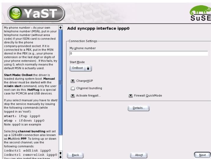
*Figure 3.21: ISDN Interface Configuration*
