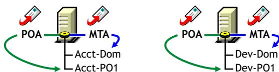
Running the POA on a remote server allows you to place the heaviest processing load on your highest performing server. In the following diagram, the agent software is installed on a different server from where the domains and post offices reside.
